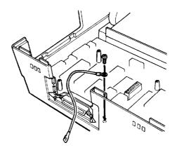
2. Carefully insert **the** pins on the optional interface board into the mating connector on the main board; then secure the board with three of the screws provided.
